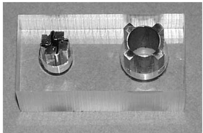
**Fig. 4** Cross-section of fixion nail – before and after inflation
